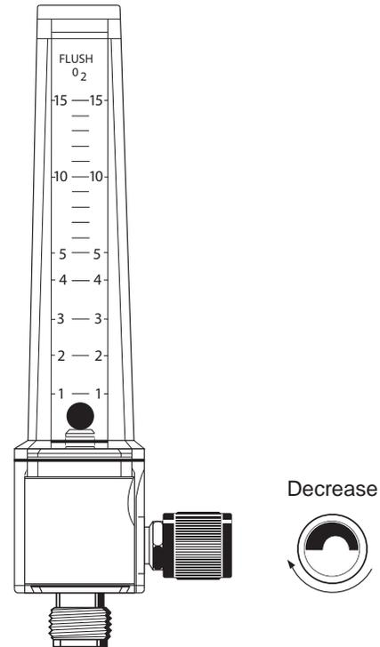
2. Rotate the flow control knob counter-clockwise (increase). The ball should rise immediately after rotation is begun, and rise smoothly and steadily with continued clockwise rotation of the flow control knob. When a desired flow is set, the ball should maintain a steady position.
