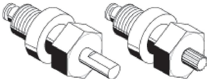
**Note:** If the flowmeter has a knurled flow control valve shaft it must be replaced by a new flow control valve assembly. Remove by following steps 4 and 5.
