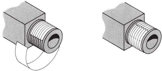
Apply Teflon tape around all pipe threads. Wrap the tape clockwise, starting one thread up, as viewed from the end of the male fitting. Apply enough pressure so the tape just starts to follow the contours of the threads. Wrap two layers of tape.
