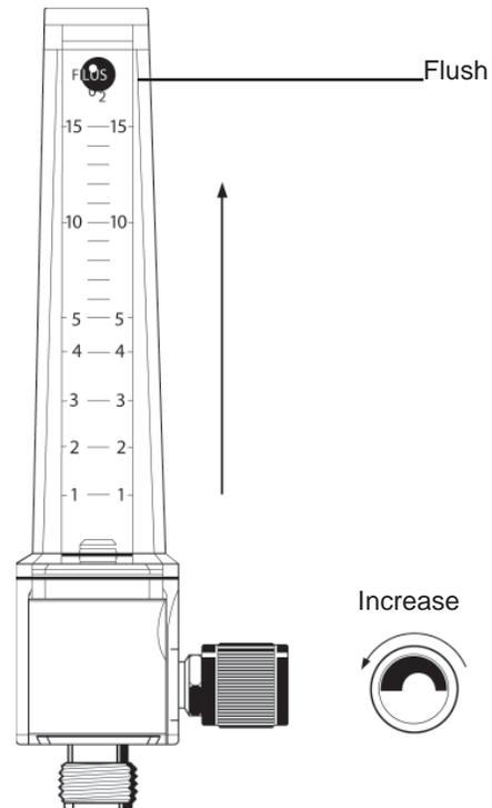
4. Rotate the flow control knob clockwise (decrease) to shut off the flow.
