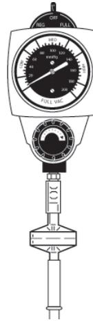
**Disposable Suction Filter on Tubing Nipple of Overflow Safety Trap**
