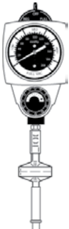
Disposable Suction Filter on Tubing Nipple of Regulator
