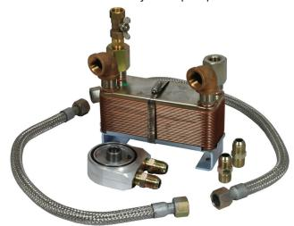
Liquid cooling kits are available for pumps located in high heat environments. The kits include a liquid to liquid heat exchanger, filter adapter plate, oil lines, fittings, and mounting hardware. Two kits handle all size pumps up to 25 HP.
